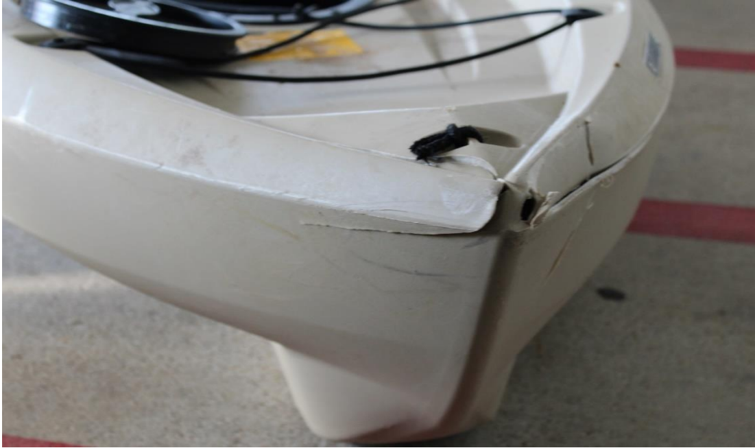
Figure 5: Damage to stern of the recreational kayak. (Unknown Date/APPD)
